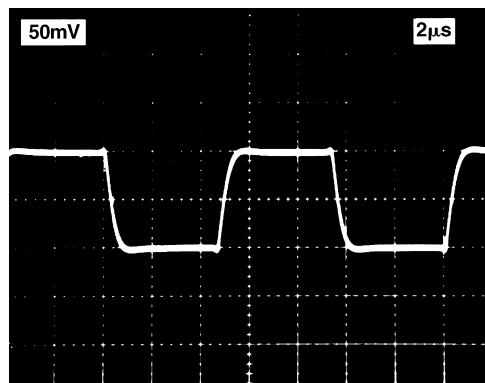
Figure 3b. Inverting Step Response
